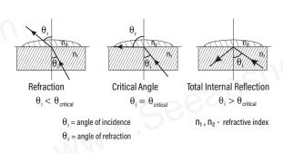
In the **MA886** refractometer, light from an LED passes through a prism in contact with the sample. An image sensor determines the critical angle at which the light is no longer refracted through the sample.
