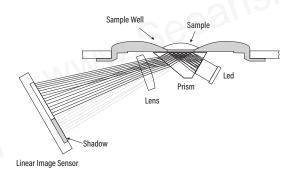
Specialized algorithms then apply temperature compensation to the measurement and convert this refractive index to: g/100 g (% by mass), g/100 mL, Specific Gravity (S.G. 20/20), or Baumé.
